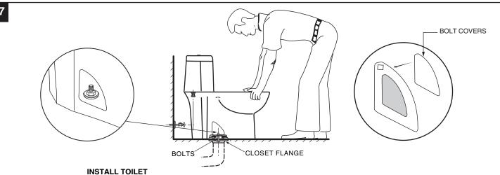
a. Position toilet squarely to wall and, with a rocking motion, press bowl down fully on wax ring and flange. Alternately tighten nuts until toilet is firmly seated on floor.
