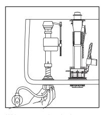
With correct washers in place (see Step 8a), tighten COUPLING NUT 1/4 turn beyond hand tight. DO NOT OVERTIGHTEN.
