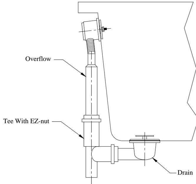
**STEP 3.** Mount handle adaptor and snap on turn handle to bath. For brass handle installation use 5/32" hex key. Adjust pop-up to min. 1/2" opening. See diagram below.
