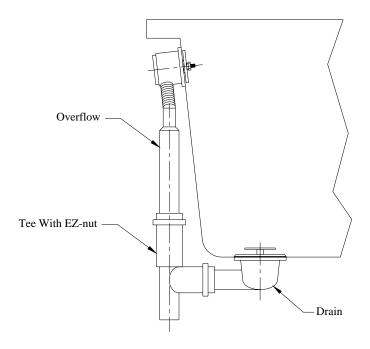
**STEP 3.** Mount handle adapter and snap on turn handle to bath. For brass handle installation use 5/32" hex key. Adjust pop-up to min. 1/2" opening. See diagram below.
